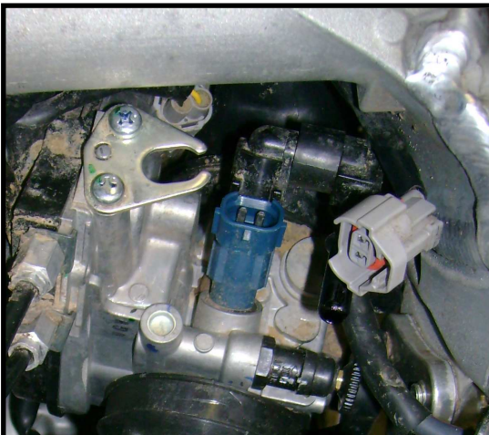
1. Detach the connector from the injector
