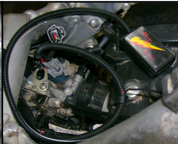
2. Place the EFI box between the original connectors
