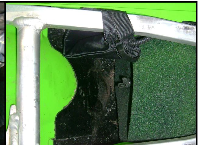
4. Place the EFI box in the bag in the air filter house
