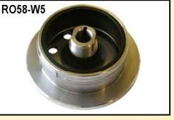
RO58-W5 YAMAHA: YZ450F (06 on) (Weighted rotor, +5ozs)
