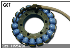
G07 Size: 115/54/26 Fits Honda, Suzuki, Yamaha, Muz & BMW motorcycles. See website for more information.
