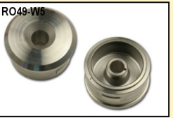
RO49-W5 KTM: SXF Models (Weighted rotor, +5ozs)
