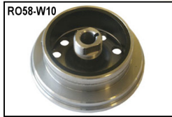
RO58-W10 YAMAHA: YZ450F (06 on) (Weighted rotor, +10ozs)
