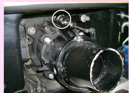
This electronic device is a replacement for the Drive & Propulsion System (DPS) of Sea-Doo Bombardier jetski's with electronic VTS.
