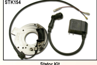
STK154 Stator Kit • Ignition only (lighting available on STK154L) • Uses original rotor/flywheel • Replaces original points system with CDI electronic ignition • Strong, reliable spark BULTACO: Sherpa Trials
