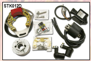
STK012D Internal Rotor Kit - Twin Spark Plug System • Digital version - Ignition only (no lighting) • Self generating CDI ignition system (no battery required) • Replaces the original Lucas alternator • Points and distributor are not required TRIUMPH: 3TA, 5TA, Unit 650 BSA: A65
