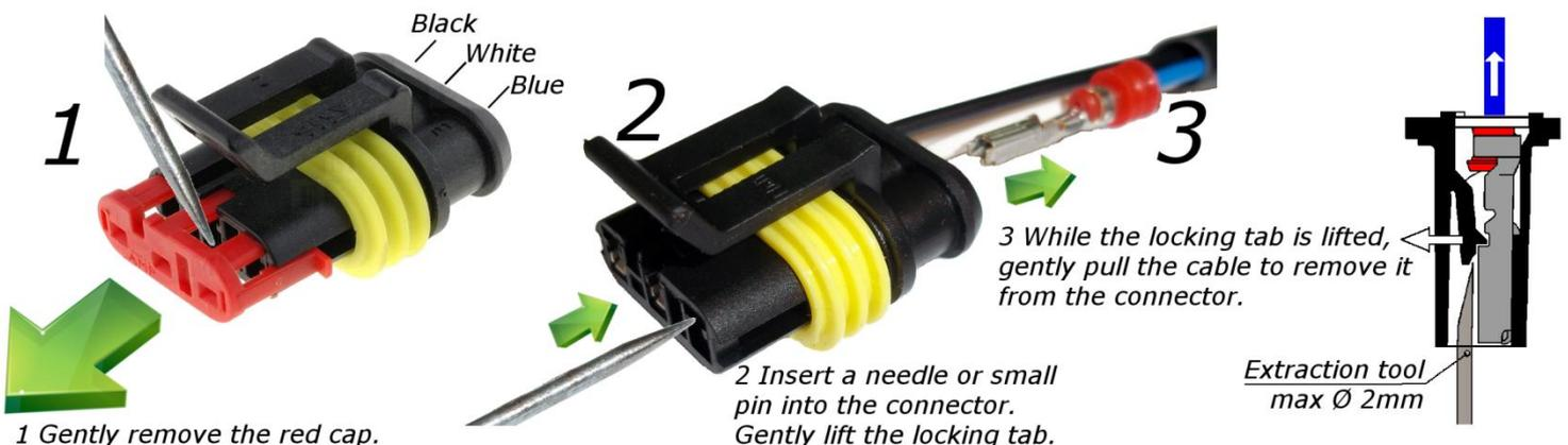
To reassemble the plug, insert the terminals back in place till the locking tab clicks in and put back the red cap.
